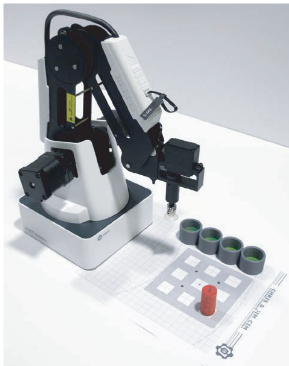
Dip Tank Set Up using 3D printed dip tanks and a Dobot Field Diagram. In this diagram four tanks are used.
