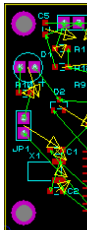
Mounting holes placed
