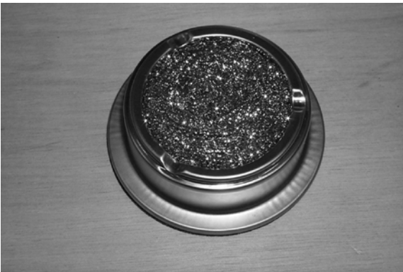
Figure 19.25 A soldering iron bit cleaner. Regular cleaning is essential to ensure good soldered joints
