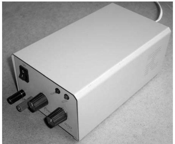
Figure 19.50 External view of the bench power supply showing the front panel controls and enclosure
