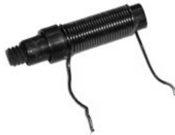
Figure 2.43 An adjustable ferrite cored inductor
