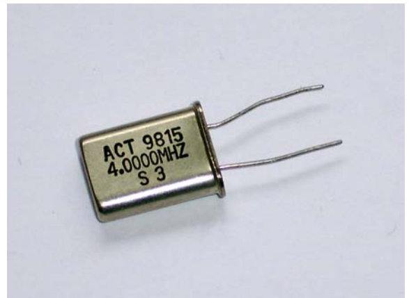
Figure 9.11 A quartz crystal (this crystal is cut to be resonant at 4 MHz and is supplied in an HC18 wire-ended package)
