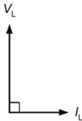
Figure 4.10 Phasor diagram for a pure inductor
